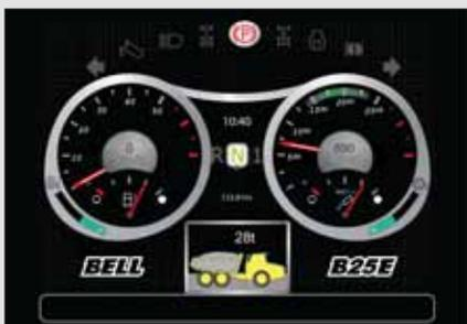
The exclusive on-board weighing option presents the operator with real time information on the payload while the machine is being loaded. A 'speed restriction' mode can also be activated if the machine is significantly overloaded.
