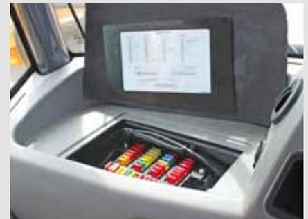
An in-cab load centre simplifies fuse replacement. Fewer relays, connectors and harnesses mean higher reliability.
