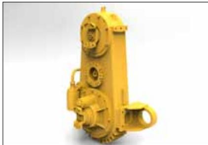
The transfer case inter-axle differential delivers equal torque to each axle when traction is favorable. When conditions deteriorate, the diff-lock automatically engages to deliver torque to the tires that can best use it.
