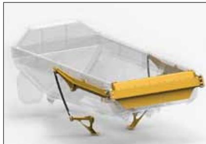
A tailgate is available as an option for better material retention. The tailgate opens as the bin is raised for dumping. Spring steel straps maintain positive seal throughout the haul, ensuring minimal material is lost.
