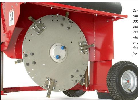
Driven by triple v-belts, the cutter wheel rotates up to 800 rpm for fast, clean cutting. A slip clutch is built into the hub of the cutter wheel, protecting the engine and drive train from wear or damage. Trench width sizes from 1"-4", depending upon model, are obtained through
