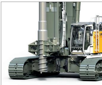
Full displacement tool with auger guide
