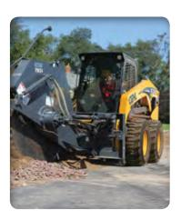
AUXILIARY HYDRAULICS are standard, powering many attachments.
