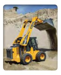
**VERTICAL-LIFT** boom design delivers extended reach and high lift heights for easy truck loading and material handling.
