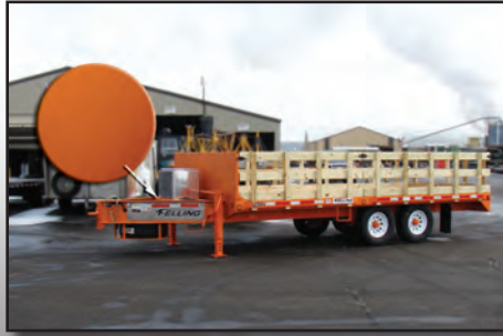
Spray-on Corrosion Liner w/ Paint
