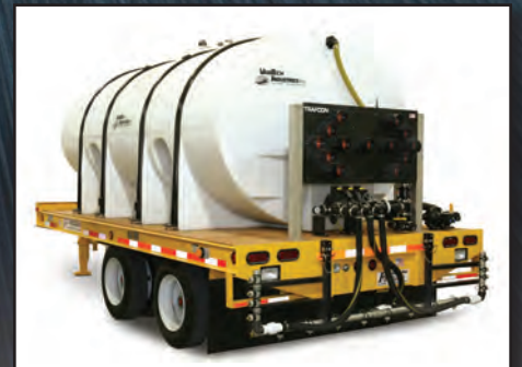
Custom Straight Deck built to be mounted with Customer's salt/ice spraying systems.
