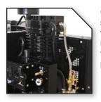
Quality cast iron two stage compressor with venting system for reduced crankcase temperature and pressure
