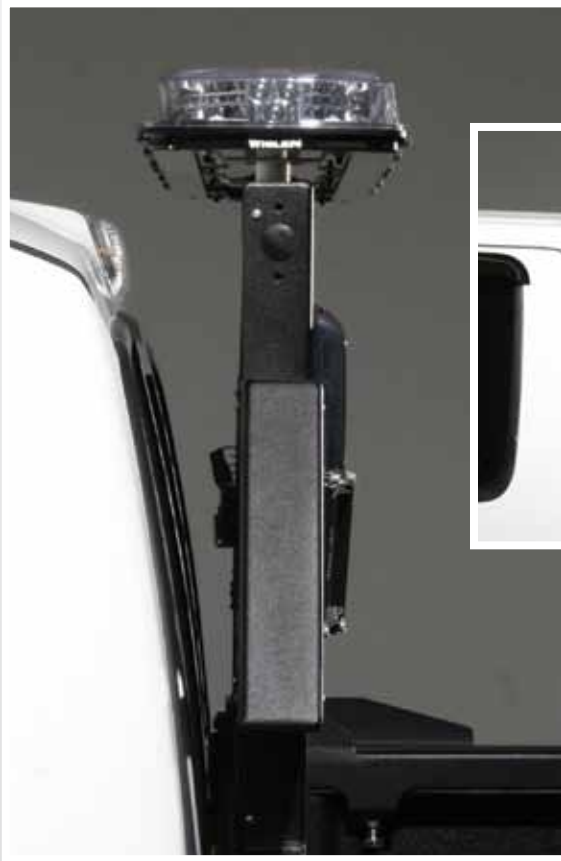
Slim design takes up minimal bed cargo space. Mounts warning light above truck cab for maximum visibility. Shown with Century Lightbar.
