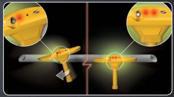
While the left or right target indicator is activated, rotate the AML until both LED target indicators light simultaneously, triggering the AML's tone and laser marker. This alert indicates that the pipe or object has been detected and that the AML is now parallel with the underground object
