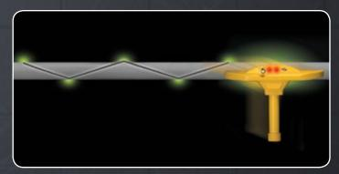
With the AML in parallel with the pipe or underground object, you can now scan the entire length of the object's edge. As an alternative, utilize the "W" method of scanning by sweeping the area in a back-and-forth "W" motion, marking the object's location and run direction as it is tracked.
