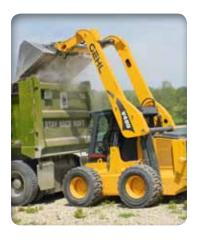
**TRUE VERTICAL-LIFT** boom design delivers extended reach and high lift heights for easy truck loading and material handling.
