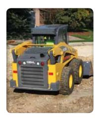
provides excellent weight distribution, enhancing machine stability. A rear bumper and counterweight on the model V330 add protection and towing capability.
