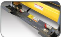
Power-A-Tach® system option allows users to quickly install and remove attachments. An operator leaves the
