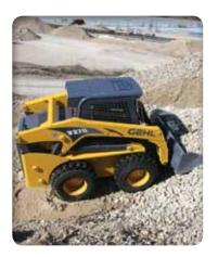
extra Long wheelbase of up to 55 inches (1387 mm) enhances machine stability when lifting and loading and provides a smoother ride over rough terrain.
