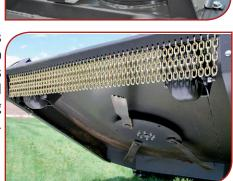
Optional dual wheel kits are available that mount to the underside of the front deck to keep the blades off the ground and prevent scalping.
