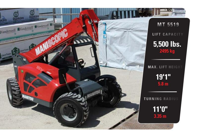
Although it's modest in size, the all-new, MT 5519 telescopic handler is the right machine when there's demanding work to be done in small spaces. With a lift height of 19'1" (5.8 m) and a maximum load capacity of 5,500 pounds (2495 kg), this machine will deliver big results in confined spaces.
