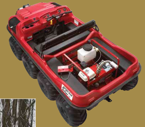
ARGO 8x8 750 HDi with spraying equipment for insect abatement
