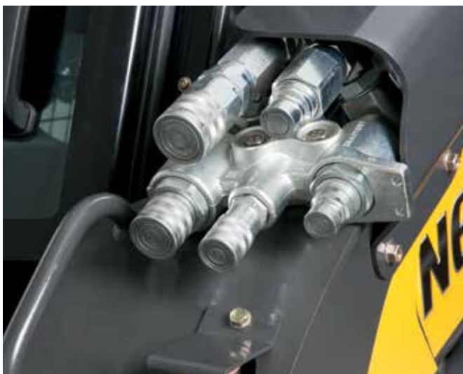
Optional high-flow hydraulics are available on the L218, L220, L223, L225, L230, C227, C232, C238.
