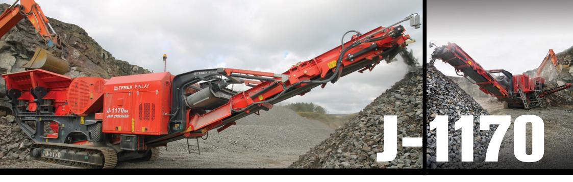
The Terex Finlay J-1170 is a compact and aggressive tracked primary jaw crusher. The heartbeat of the machine is a robust hydrostatically driven Terex jaw chamber which provides high capacity with large reduction ratios. The jaw chamber configuration can be set up specifically for quarrying applications or processing construction demolition debris using the hydraulic release chamber option.
