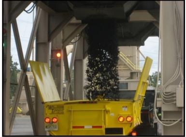
3-Ton Trailer Loading at the Asphalt Plant
