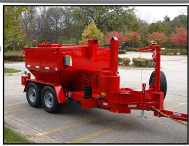
4-Ton Trailer with Dual Burner Recycling Package, Heated Tack Tank with Pour Pot, Tool Holder, Compactor Basket, ST235/80-R 16" Tires and Hoist
