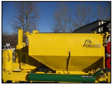
5-Ton Dual Burner Slip-in with Heated Tack Tank and Other Options
