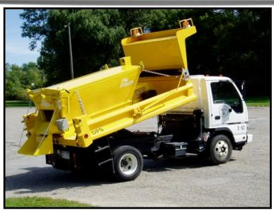
2-Ton Slip-in Mounted on Dump Bed
