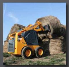
operate safely with clear side and rear sight lines for full, expansive views for increased safety and precision placement. A roof grid section provides visibility to the bucket at full lift height.
