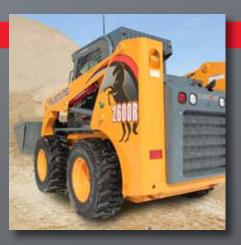
SMOOTH RIDE ▲ is achieved with a longer wheelbase and low center-of-gravity. The HydraGlide<sup>™</sup> ride control option provides stable operation over uneven surfaces.
