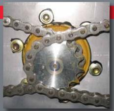
HEAVY-DUTY DRIVETRAIN ▲ is composed of durable components, including zero-maintenance axles. Adjustments can be made to the chain system from outside the unit.
