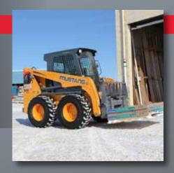
SPEED UP ▲ with maintenancefree, radial-piston drive motors with high start-up torque and maximum ground speeds up to 12.5 mph¹ (20 km/hr) for quick acceleration.
