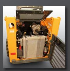
QUICK SERVICE A is made possible with a swing-open rear door, flip-up engine cover, and tiltable ROPS/FOPS that fully exposes maintenance points at the engine, battery, and filler caps.
