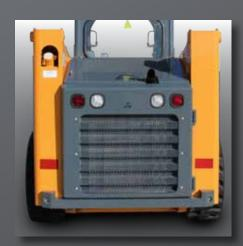
counterweights are optional and boost the rated load capacity to 2,110 lbs. (957 kg) on the 1900R, 2,370 lbs. (1075 kg) on the 2200R, and an impressive 2,780 lbs. (1261 kg) on the 2600R.
