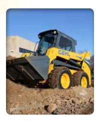
**STABLE RIDE** is achieved with a longer wheelbase and low center-of-gravity. The HydraGlide<sup>TM</sup> ride control option provides smoother operation over uneven surfaces.
