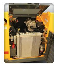
SPEEDY SERVICE is made possible with with a swing-open rear door, flip-up engine cover, and tiltable ROPS/FOPS that fully exposes maintenance points at the engine, battery, and filler caps.
