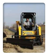
ACCELERATE RAPIDLY with maintenance-free, radial-piston drive motors with high start-up torque and maximum ground speeds up to 12.5 mph<sup>1</sup> (20 km/hr).
