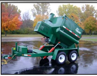
4-Ton Dump Box with Winterization Package and Dual Burner Recycling Package
