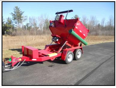
2-Ton Dump Box with Arrow Stick, 24-Hour Timer and Hydraulic Doors
