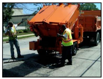
4-Ton Dump Box with Tack Tank, Solvent Tank and Hydraulic Doors Offloading Recycled Asphalt
