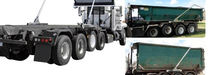
bumpers on bow contact the rear of the container. After the adjustable tower is lowered, the tarp can be 'winched' onto the container to provide a snug overall fit.
