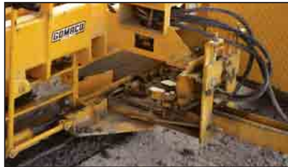
Female keyway with hydraulic side bar insertion and vibration to the bar.
