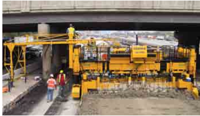
The gantry system on the GHP-2800 is hydraulically extended, and normal paving continues once the paver is clear of the bridge piers under the overpass.
