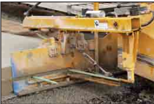
Sideplate Extension With Air-Powered Bar Insertion. GOMACO's air-powered bar insertion will accommodate most types of bars.
