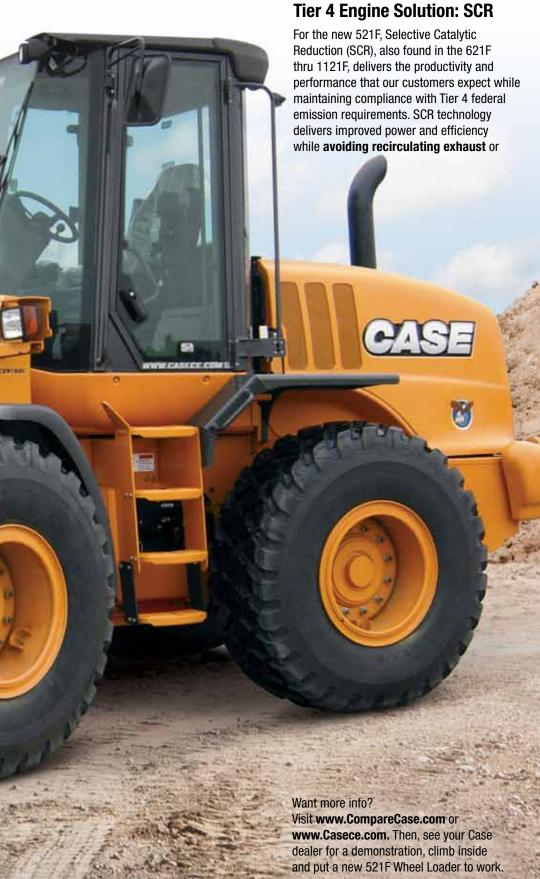
costly regenerative cycling. Also, due to the avoidance of high exhaust temperatures, the 521F can operate in a wider variety of applications. With the Case SCR's simplified design, there are fewer components and service issues to address.
