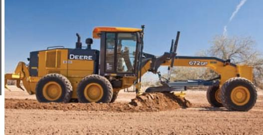
GPS+ and MMGPS+ systems work extremely well when machines are capable of receiving GPS satellite signals, but what happens when the jobsite does not have visibility to open sky? Working between buildings or in heavy tree coverage can limit the performance of a 3D-GPS control machine. In these situations Topcon's LPS-900 (Local Positioning System) is the ideal system for guiding your machines.
