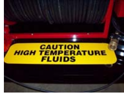
“Hot Fluid” on deck below hose reel
