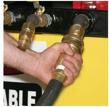
Attach 1" male disconnect to return.
