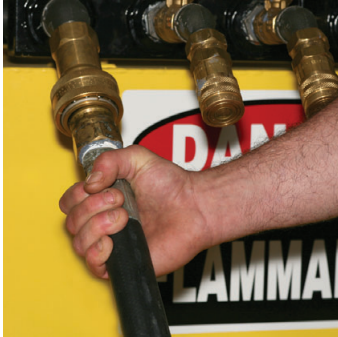
Attach 1" female disconnect to supply.
