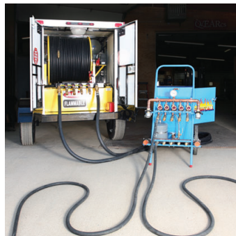
When all connections are complete, this is how the equipment should appear. NOTE: This photo denotes the use of only ONE loop.
