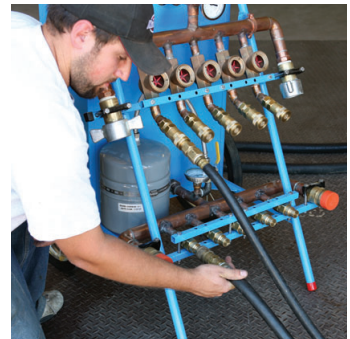
Lay out hose in configuration needed. Connect secondary hose to CCS supply. Repeat previous #8 and this step #9 for additional hose loops.
