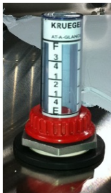
35: HTF Level Gauge
