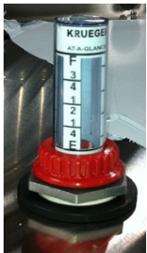
35: HTF Level Gauge
