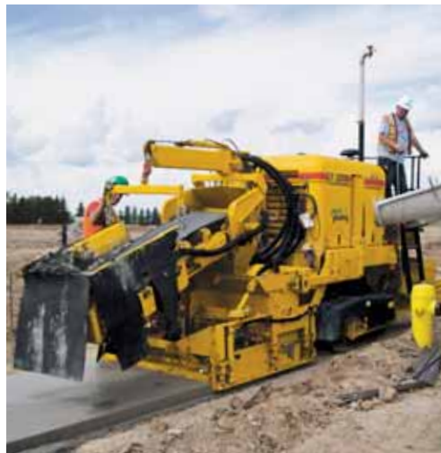
The hydraulic swinging conveyor can be moved in order to avoid obstacles while paving.
