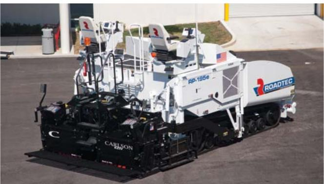
The RP-195e is a powerful, heavy-duty rubber-track paver for highway work offering operator comfort and safety with 360° visibility, fingertip controls, fully adjustable seats, low noise levels, and fume extraction systems. The exclusive Roadtec anti-segregation design gives consistent pavement quality. Dependable and tough.
