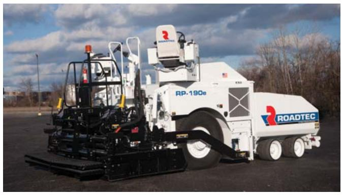
The RP-190e is a powerful, heavy-duty rubber tire paver for highway work offering operator comfort and safety with 360° visibility, fingertip controls, fully adjustable seats, low noise levels, and fume extraction systems. The exclusive Roadtec anti-segregation design gives consistent pavement quality. Dependable and tough.
