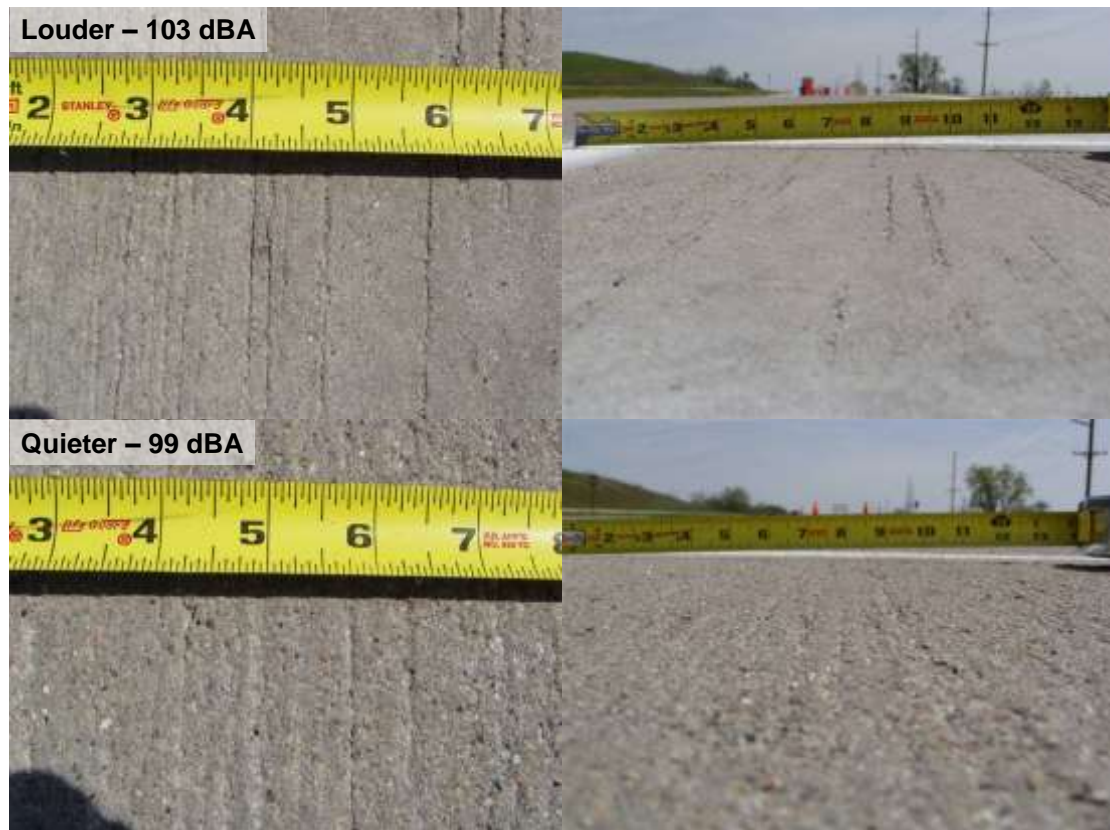
Figure 6. Variability of drag texture surface and its effect on OBSI noise level.
