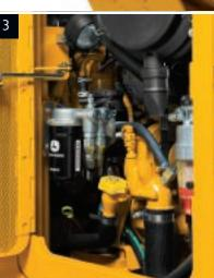
To help conserve fuel and comply with regional regulations, auto-shutdown automatically turns off the engine after an operator-determined period of inactivity. The swing-out side shields and tilt-out grille provide access to both sides of coolers for easy cleaning. Hydraulically driven ondemand fan runs only as needed, reducing fuel consumption and wear-causing debris flow through the cores.
