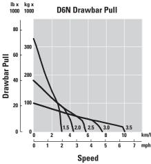
The direct injection electronic fuel system provides a controlled fuel delivery increase as the engine lugs back from rated speed. This results in increased horsepower below rated power. A combination of increased torque rise and maximum horsepower improves response, provides greater drawbar pull and faster dozing cycles.
