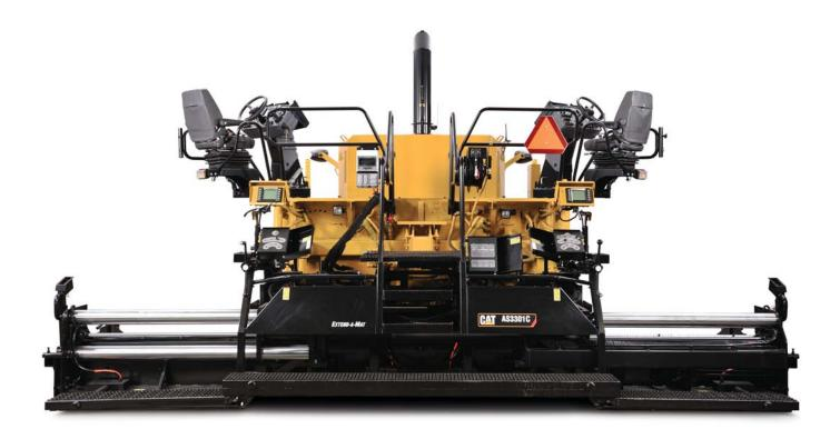
Heavy-duty support tubes stabilize the extenders providing even material flow for high quality results on interstates, highways, airports and other high-production paving applications.
