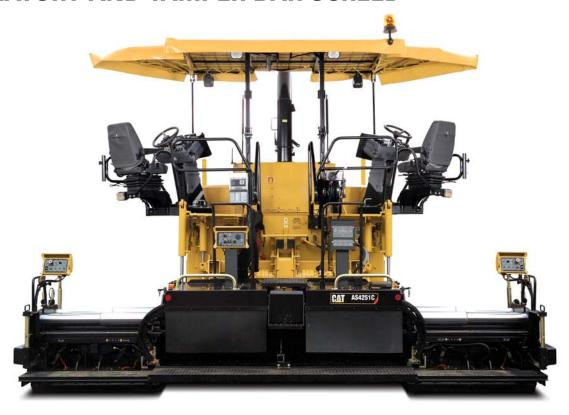
Tamper bars combined with vibratory screed plates optimize mat density behind the screed.
