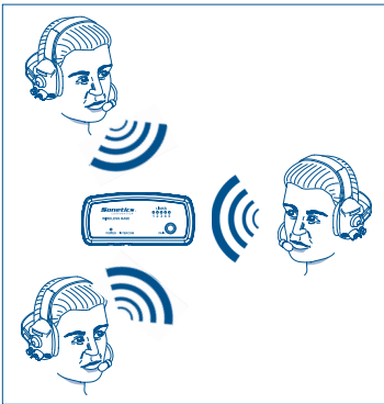
Figure 1 Basic, single-site wireless team communication system
